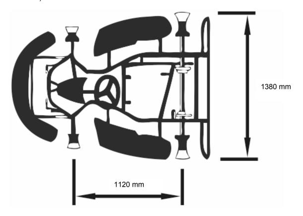
(a) The tyres on the go-kart have an outside diameter of 460 mm. This makes the ratio of the rear axle height to width equal to 6:1.
