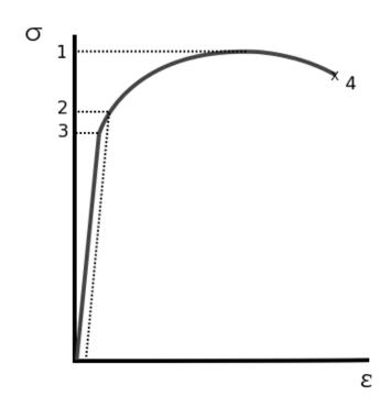
(g) During a tensile test of the aluminium tie-rod, a stress-strain graph was plotted similar to the one shown above. Identifiable regions and/or points on a stress-strain graph include the following: fracture; elastic deformation; plastic deformation; proportional limit; tensile strength; yield strength. Use this list and your Engineering knowledge to name the numbered points on the graph. (4 marks)
