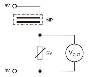
(i) Calculate the output voltage ( $V_{OUT}$ ). Assume the resistance of MP (moisture probe) is 50 k $\Omega$  and RV is set to 12 k $\Omega$ . (3 marks)
