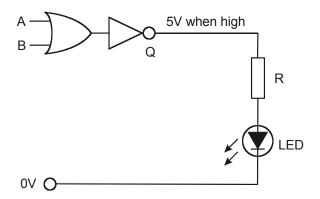
Calculate the ideal value for the series resistor that would be used with the LED.
