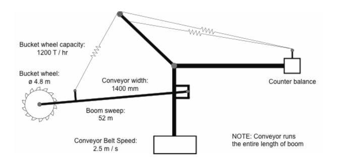
(a) Each bucket on the bucket wheel reclaimer has a capacity of 500 kg of crushed ore. Calculate the maximum rise in potential energy of a single bucket as the wheel rotates.
